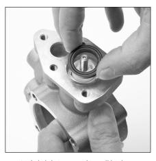
6.11 Lightly lubricate and install high pressure seal (22) with metal backing facing down over ceramic plunger (21).
