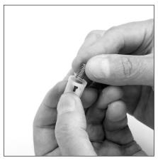
6.17 Assemble the discharge valve as follows: Insert spring (26) into retainer (27).
