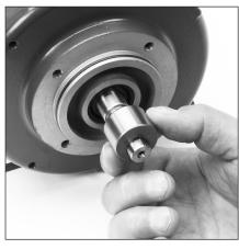
6.5 Lubricate and install cam (8) over motor shaft and key. Position cam (8) so stamped cam ID number is facing
