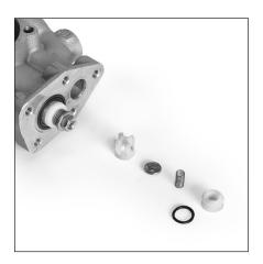
5.12 Separate and inspect retainer (27), spring (26), valve (25), seat (24), and o-ring (23).
