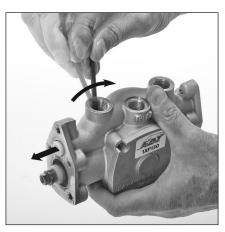
5.11 Pivot 5M allen wrench against top of spring retainer and push valve assembly out.
