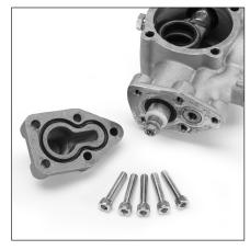
5.9 Use a 5mm allen wrench to remove five (5) M6x30 screws (13) holding head cover (14) to crankcase body.
