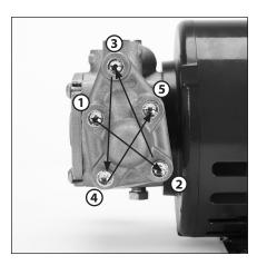
6.24 Use a 5mm allen wrench to torque to 102 in-lbs in sequence as shown.
