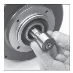
5.5 Remove and inspect cam (8) from motor shaft.
