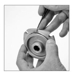
6.7 Lubricate and install o-ring (6) onto bearing cover (5).
