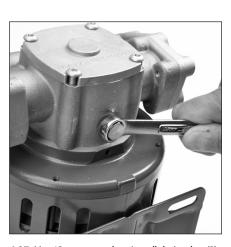
6.27 Use 13mm wrench to install drain plug (3) into bottom port of crankcase body (1).
