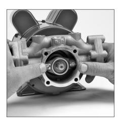
6.25 With bearing cover (5) removed, position crankcase body (1) onto motor while lining up the connecting rods (28) with the cam (8).
