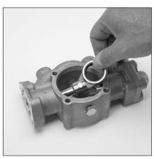
5.15 Remove and inspect connecting rod, plunger rod and wrist pin assembly.
