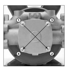
6.26 Hand thread four (4) M6x75 button head screws (4). Use a 4mm allen wrench to torque to 48 in-lbs in sequence as shown.
