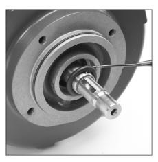
5.8 Use a pick tool to remove slinger o-ring (11) from motor flange.
