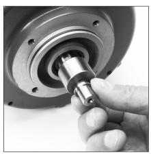
6.6 Install retaining ring (7) into snap ring groove on motor shaft to secure cam (8).
