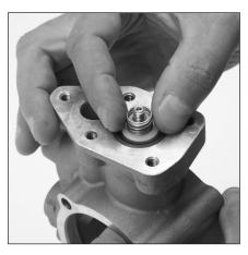
6.14 Install spring (18) over spacer (19) and on to inlet valve (20).
