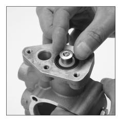
6.15 Install washer (17) with curved surface down on to spring (18).
