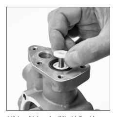
6.12 Install inlet valve (20) with flat side down onto plunger (21).
