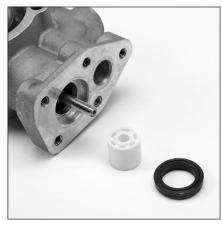
5.14 Remove and inspect ceramic plunger (21) and high pressure seal (22) from crankcase body (1).
