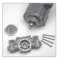
5.3 Use a 4mm allen wrench to seperate pump (1) from motor (2) by removing four (4) M6x75 button head screws (4) from bearing cover (5).
