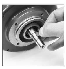
6.4 Lubricate and install woodruff key (9) into motor shaft keyway.
