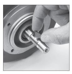
5.6 Remove and inspect woodruff key (9) from keyway of motor shaft.
