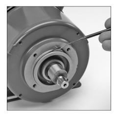
6.3 Lubricate and install o-ring (12) onto motor flange.
