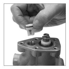
6.21 Press discharge valve assembly (30) into top hole with retainer facing into crankcase body (1) until flush with cylinder head surface.
